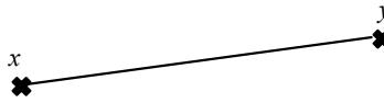
Figure 3: All convex combinations z = \theta x + (1 - \theta)y of two points x and y lie on the line segment from x to y . When \theta = 1 , we get x and when \theta = 0 , we get y .
